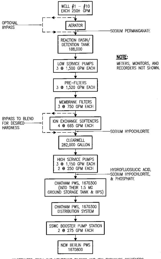
WASTEWATER FROM THE MEMBRANE FILTERS AND ION EXCHANGE SOFTENERS IS DISCHARGED TO TWO LAGOONS AND ONE WASTEWATER TANK.
